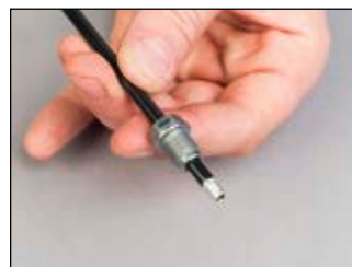
Mounting the union nut
