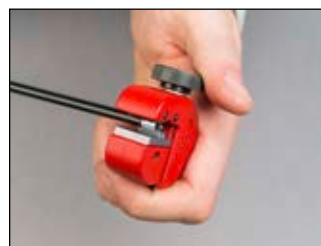
Positioning of line to scrape the covering
